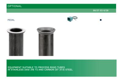
This machine, which requires only one tool change to carry out the flaring operations, uses a cold orbital forming process to create a flat and smooth sealing surface at 90° and 37° with a suitable rugosity for the O-Ring seal. The innovative clamping system enables to process straight and of reduced dimensions rigid tubes, so this machine is the ideal solution for tubes with bends up to 180° with a tight radius, such as shaped rigid tubes, steel and hose combined connections, etc.
