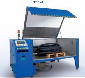
WITH PNEUMO-HYDRAULIC MULTIPLIER; IDEAL FOR PALLETISED HOSE COILS
